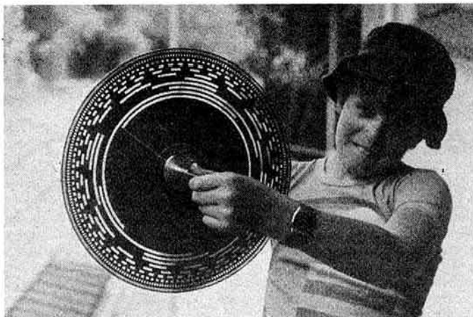
Gray code shaft encoder used by Z25JJ to provide high accuracy indication of elevation and azimuth of his 32ft dish
